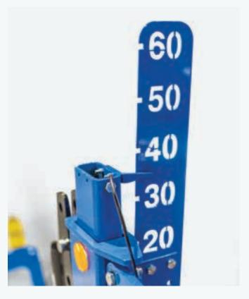
A graduated scale, easily visible from the tractor cab, provides an indication of the set working depth.
