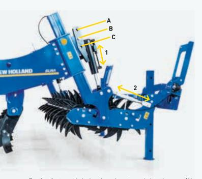
Depth adjustment is hydraulic and can be varied on the move (1) 3 depth ranges can also be set for:
