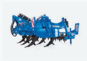
SUH subsoilers have been developed to work the most demanding soils and operate at depths of up to 550mm. Ideal for both contract operators and intensive workloads, SUH models are extremely robust. A CAT III / IV N hitch is standard.
