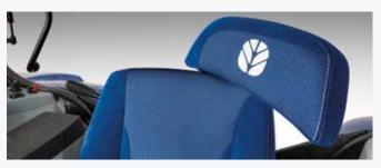
Both the Dynamic Comfort and Comfort seats benefit from the innovative swiveling backrest, designed to provide upper back support and significantly increases comfort when the seat is turned to monitor rear mounted implements.
