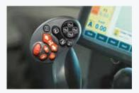
The soft-touch buttons feature backlight technology to make selecting controls in the dark even easier. Fingertip control for up to two remote valves, which can both be configured with remote valve management.
